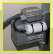
Powerful 1,5 hp motor creates minimal noise, even when cutting through 22 mm materials.
